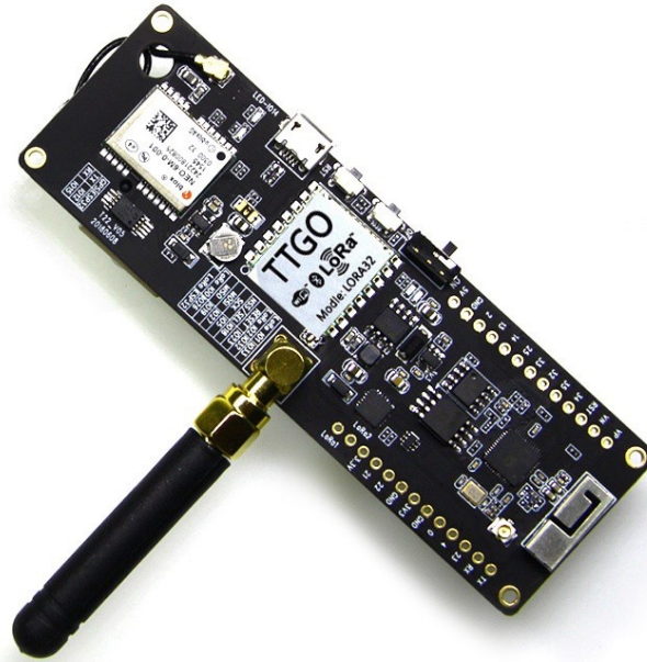
Fig. 36: TTGO T-Beam from Wemos. TTGO T-Beam pinout, example code.
