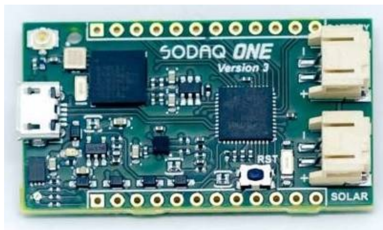
Fig. 34: SODAQ ONE-EU-RN2483-V3 from SODAQ. SODAQ ONE tutorial with explanations, schematics, datasheets, and examples. SODAQ ONE module pinout
