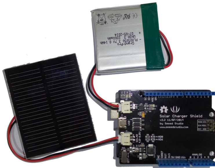
Fig. 2: Solar shield connections with the solar panel and a battery.
