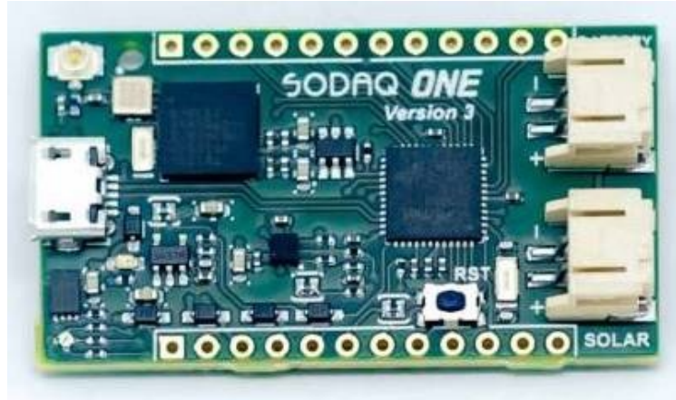
Fig. 35: SODAQ ONE-EU-RN2483-V3 from SODAQ. SODAQ ONE tutorial with explanations, schematics, datasheets, and examples. SODAQ ONE module pinout
