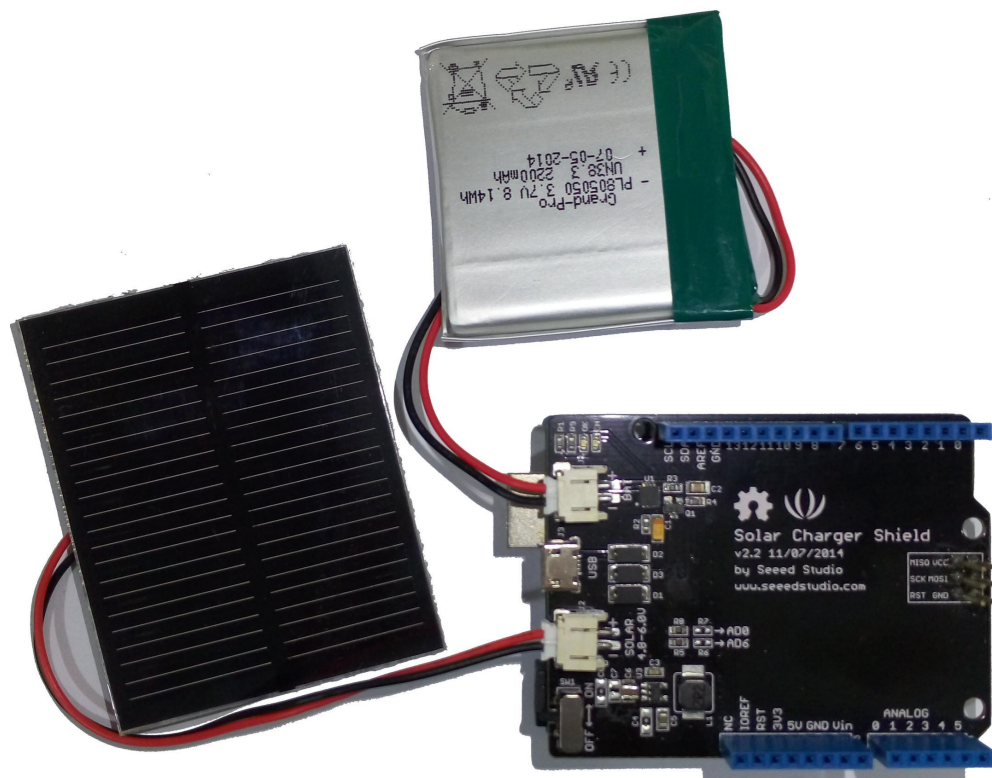
Fig. 22: Solar Charger Shield V2.2 from Seestudio.
